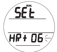
Fig. 24 - SET DUAL TIME (hour differential)
