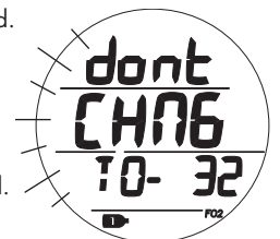
Fig. 99 - GAS SWITCH ALARM (all flash)
