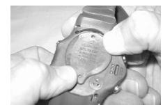
Fig. 136B - COVER INSTALL (using thumbs)
