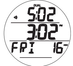
Fig. 25 - WATCH TIME (Dual Time set and On)
