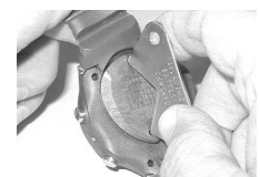
Fig. 136A - COVER INSTALL (using tool)
