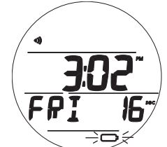
Fig. 2 - WATCH (low battery alarm)
