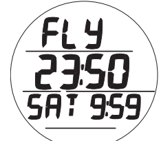
Fig. 33B - FLY/SAT (10 min after dive)
