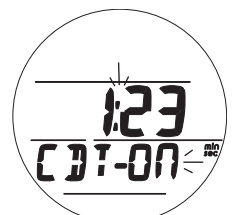
Fig. 112 - CDT STATUS (On, running)
