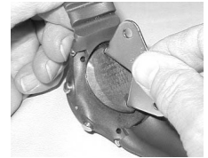
Fig. 132A - COVER REMOVAL (using tool)
