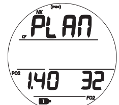
Fig. 34B - PLAN LEAD-IN (Gas 1 set for Nitrox)
