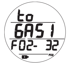
Fig. 98 - GAS 1 SWITCH PREVIEW
