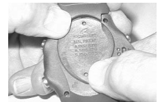
Fig. 132B - COVER REMOVAL (using thumbs)
