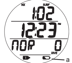
Fig. 1 - SURFACE MAIN (low battery warning)
